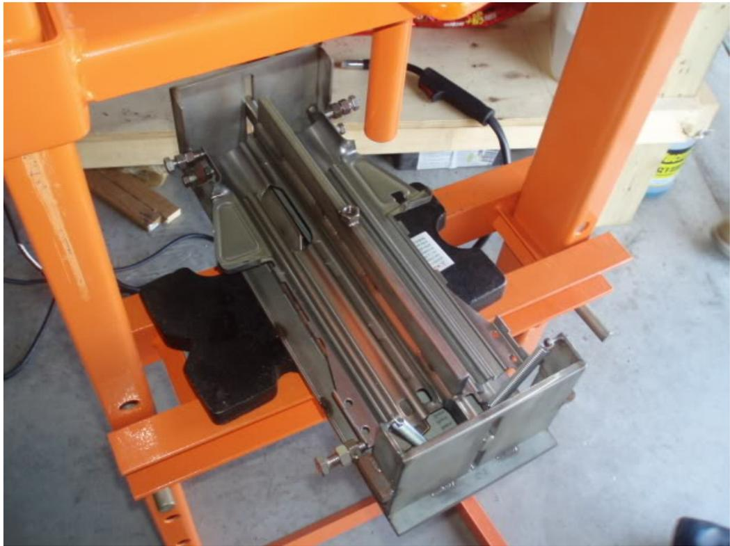
Once pressure is applied, the ends begin to rise up (if you've done an AK, you are familiar with this) and keep [applying](#) slow gentle pressure on it, and keep both ends coming up at roughly the same pace. Every flat I bent tended to rise up on the left side a bit faster than the right, but they came out just fine.
