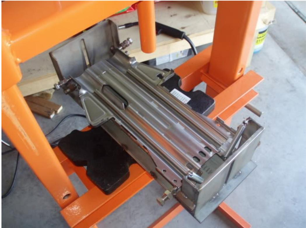
Next, put the rod piece in. This is a round bar that basically forms the top radius of the bend. It is guided by slots on the front and rear of the jig. Begin to slowly [apply](#) pressure and watch as the flat begins to slowly form up.
